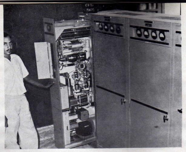
Wilcox type 96D 3 kW communications, high and low frequency, multi-channel transmitters with Indian Posts & Telegraphs Department.
