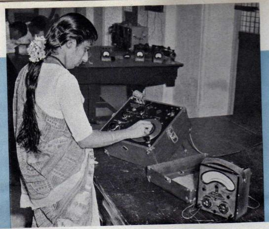
Measuring the unknown capacitance using a General Radio Capacitance Test Bridge.
