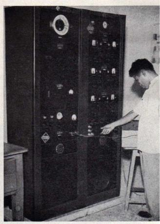
GR Standard Frequency Measuring Equipment at one of the Defence Laboratories.
